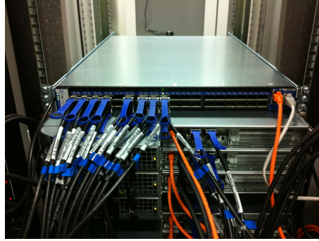
Figure 7.9: Timeslice building test setup (MicroFLES) with InfiniBand FDR switch.
