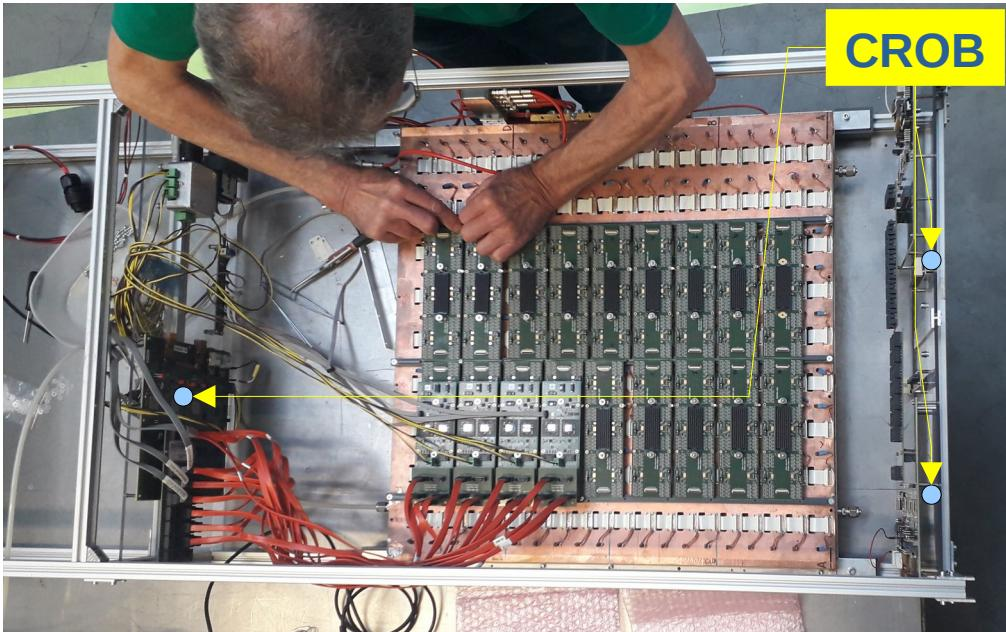
**Mounting the 14 new FASPRO boards on the TRD2D.** The operated region was modified wrt planning as follows (see picture, top to the right):
