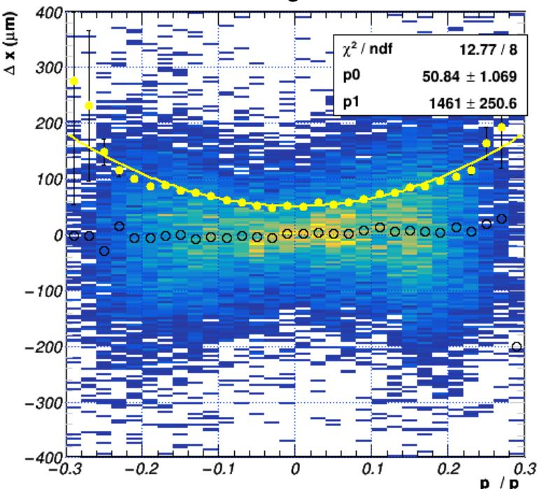
The distribution of  $\Delta x$  (residuals) between TRD2D hits and MC points as function of  $\varphi = p_x/p_z$ . The shift (black symbols) and the resolution (yellow) of each vertical slice are superimposed.
