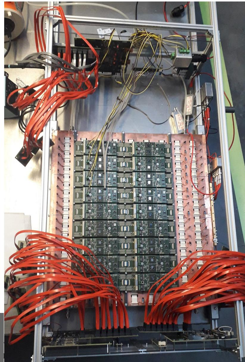
**Mounting the corresponding GETS boards.** The red cables left floating are the connections to the CROB. Due to topological reasons the allocation GETS → CROB will differ from previous runs which will impact the software mapping !
