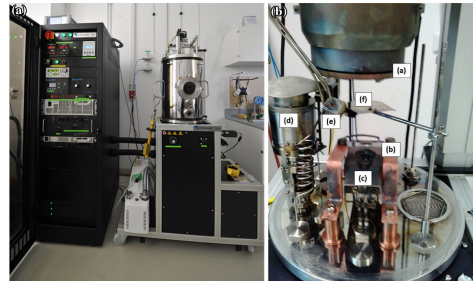
Fig. 2 A TE18-High Vacuum Deposition System produced by Intercovamex Company; B interior of the deposition chamber, showing: a rotating substrate holder; b thermal evaporation; c electron-beam evaporation system; d sputtering deposition system; e quartz crystal monitor; f shutter
