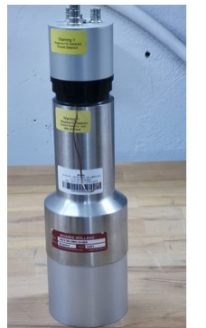
ELIGANT 3x3" \text{LaBr}_3(\text{Ce})/\text{CeBr}
