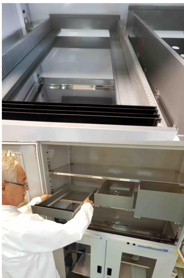
Fig.10. Left: Special boxes used to store the glass plates passing a preliminary optical QA upon arrival from producer; Right: Boxes with the glass plates in are stored in a super dry cabinet in the clean DetLab where the RPC assembling with take place.
